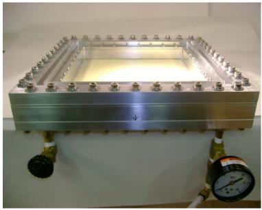
First test, at oxygen overpressure, ~ 4 cc/hour/panel.
