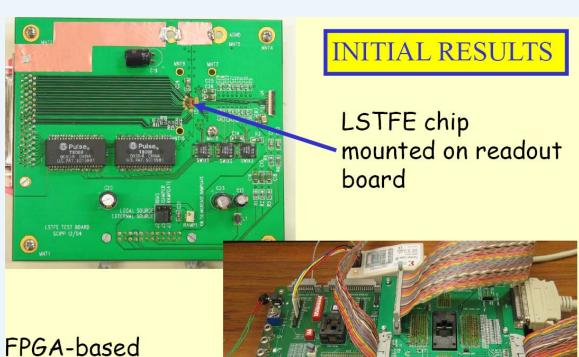
FPGA-based control and data-acquisition system
