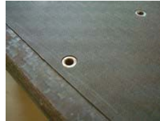
Uniform dispatch of 18 inserts on the 15mm thick plate
