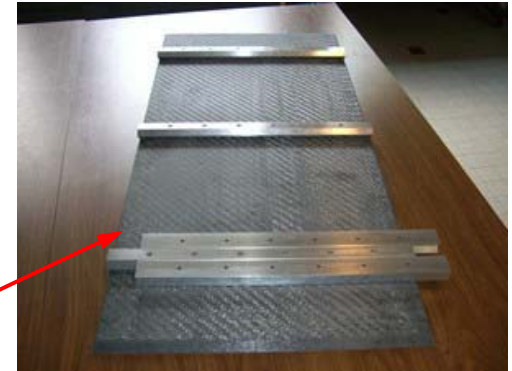
15mm thick plate with it's rails; ready to be assembled with alveoli layers
