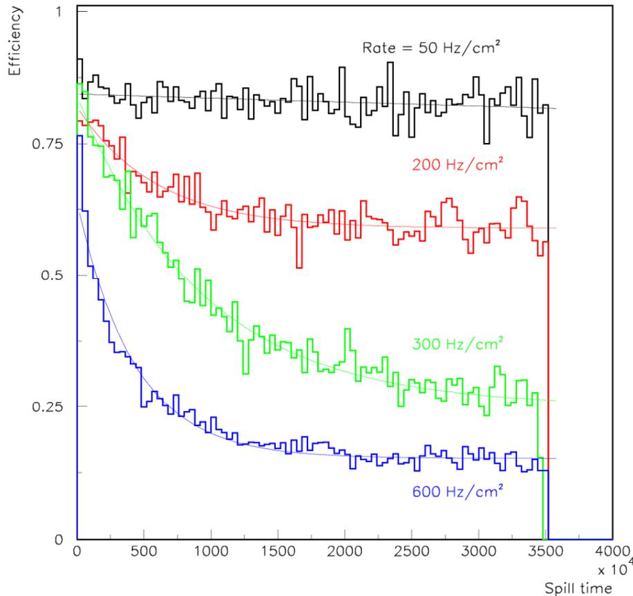
At high rate efficiency drops and then levels out
