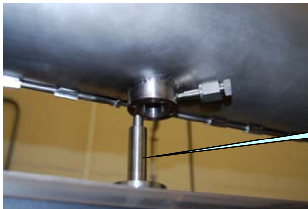
3. Cold mass securing pin
