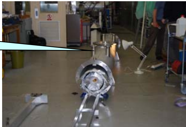
3. Cold mass and radiation shields inserted into vessel
