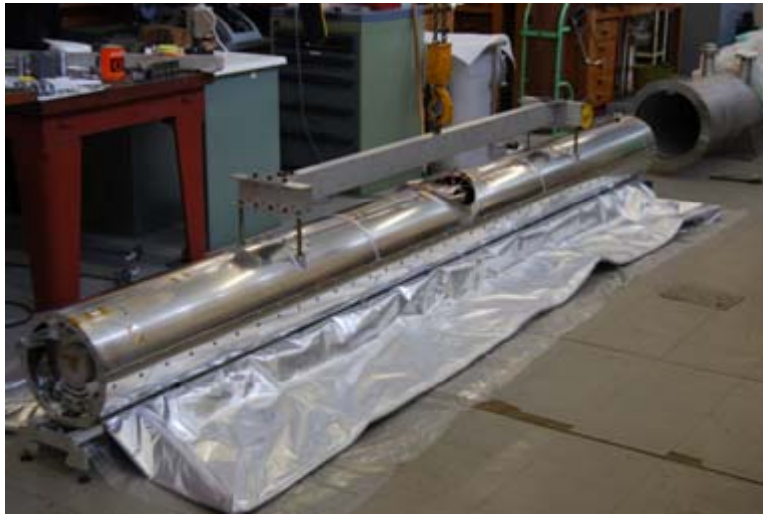
1. Mli blanket over radiation shield
