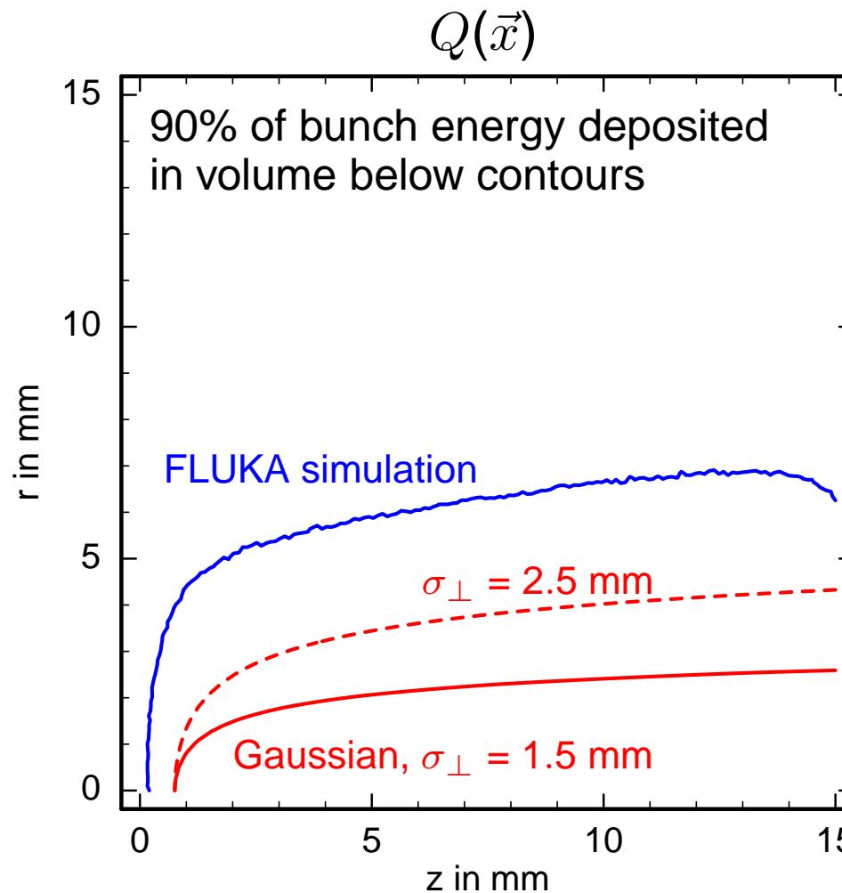
⇒ In (more realistic) FLUKA simulation the energy is distributed in larger volume than in Gaussian approximation
