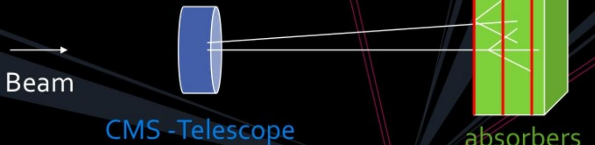
Simple case of PFA study can be achieved at low cost by combining existing/future calorimeters with existing tracker telescope
