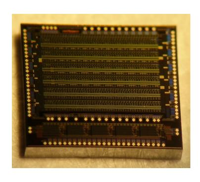
Prototype ADC channels with and without S/H fabricated in AMS 0.35  $\mu m$  technology
