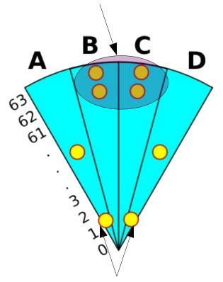
Each yellow dot means : 1 ASIC (8 channels)
