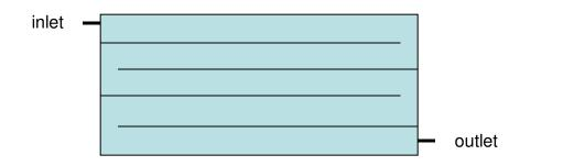
Use fishing lines both as spacers and as chicane for the gas
