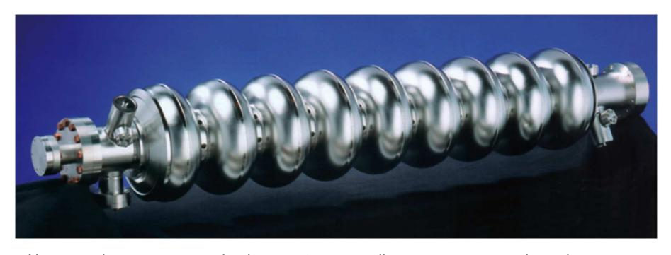
$\bullet$  About  $1\,\mathrm{m}$  long, super-conducting,  $1.3\,\mathrm{GHz}$ , standing wave, constant impedance,  $31.5\,\mathrm{MV/m}$
