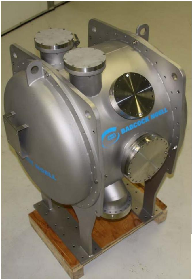
**Under construction** cold vacuum chamber for diagnostics to **measure the beam heat load** to a cold bore in a storage ring. The beam heat load is needed to specify the cooling power for the cryodesign of superconducting insertion devices.
