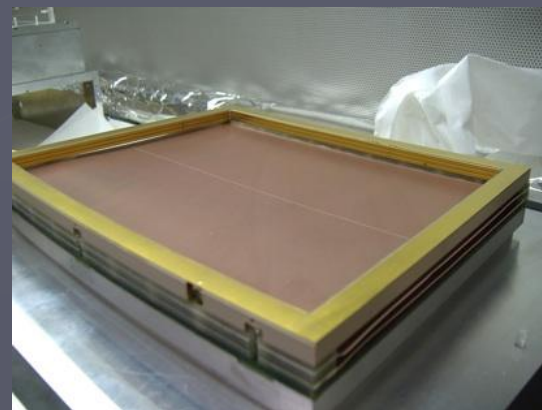
An Asian GEM modules with a field shaper in the place of the gating GEM
