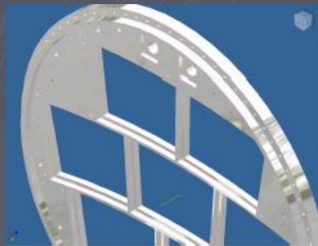
Current LP1 endplate mechanical structure
