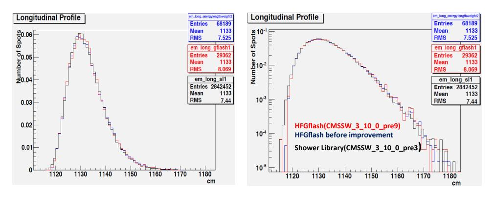
Longitudinal profile produced by 100-GeV electron gun using HFGFlash, HFGFlash 2 and Shower Library(based on Geant4)
