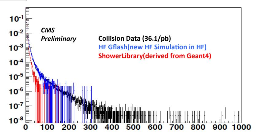
HF Gflash has better agreement to 36.1 pb-1 Certified Collision Data compared to previous simulation
