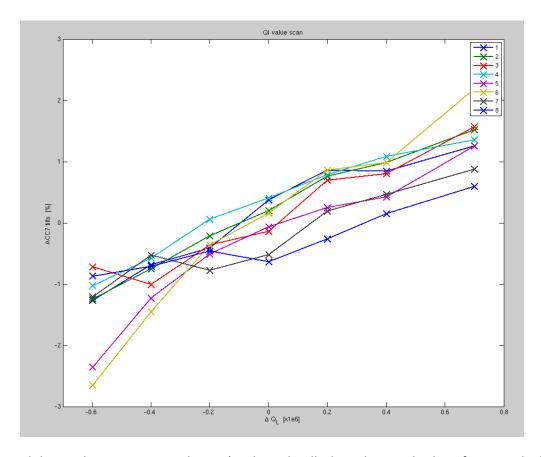
We retuned the machine to its original state (i.e. brought all QIs to the initial value of  $^{\sim}$ 3e6 and adjuted detuning).
