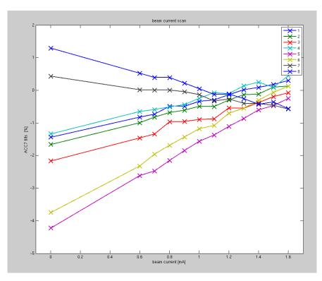
We then restore the beamloading back to 1.6nC, and scan QL up and down from the optimum value, in constant steps of 0.2e6. Again all cavities behave linearly around the optimum value and 0% tilt.
