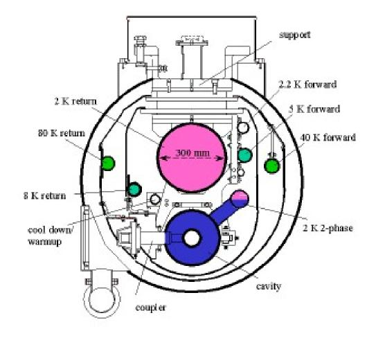
Figure 3.2.11: Cross section of cryomodule.
