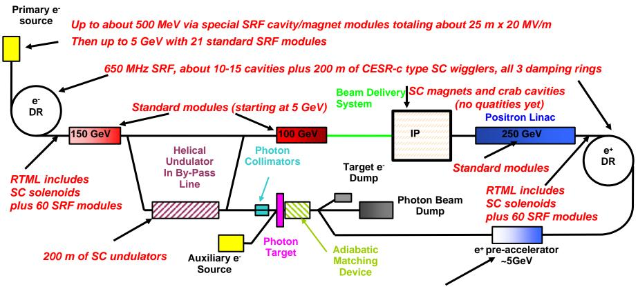
Up to about 500 MeV via special SRF cavity/magnet modules totaling about 25 m x 20 MV/m Then up to 5 GeV with 21 standard SRF modules
