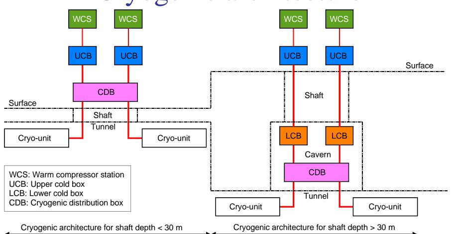
For shaft depth above 30 m, the hydrostatic head in the 2 K pumping line becomes prohibitive and active cryogenics (e.g. cold compressor system) has to be installed in caverns (LBC), i.e. additional cost for cryogenics and civil engineering. 26 LCFOA at SLAC
