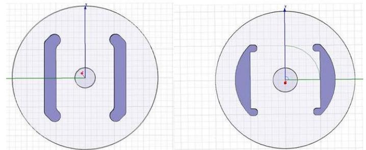
A small stripline beam pipe radius results in closer values of even and odd mode characteristic impedances.
