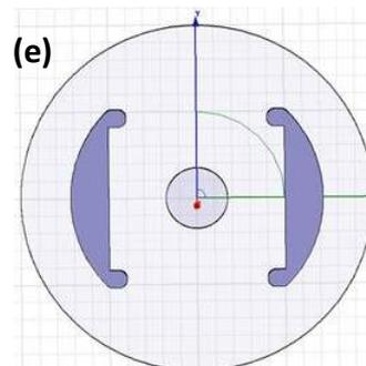
Different **half-moon electrode** shapes ((c), (d) and (e)) have been studied because with them we could keep the good field homogeneity of the flat electrodes, as well as trying to decrease the stripline beam pipe radius.
