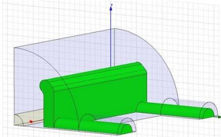
A total of four coaxial **feedthroughs**, with  $50\ \Omega$  characteristic impedance, are required to transfer power:
