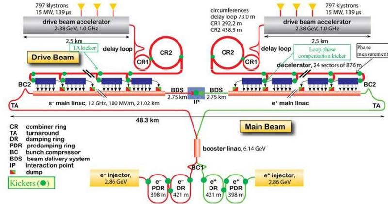
Kickers are required to inject beam into and extract beam from the PDRs and DRs for both the main beam of CLIC.
