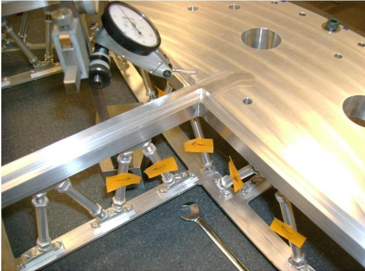
The strut design allows alignment correction.
