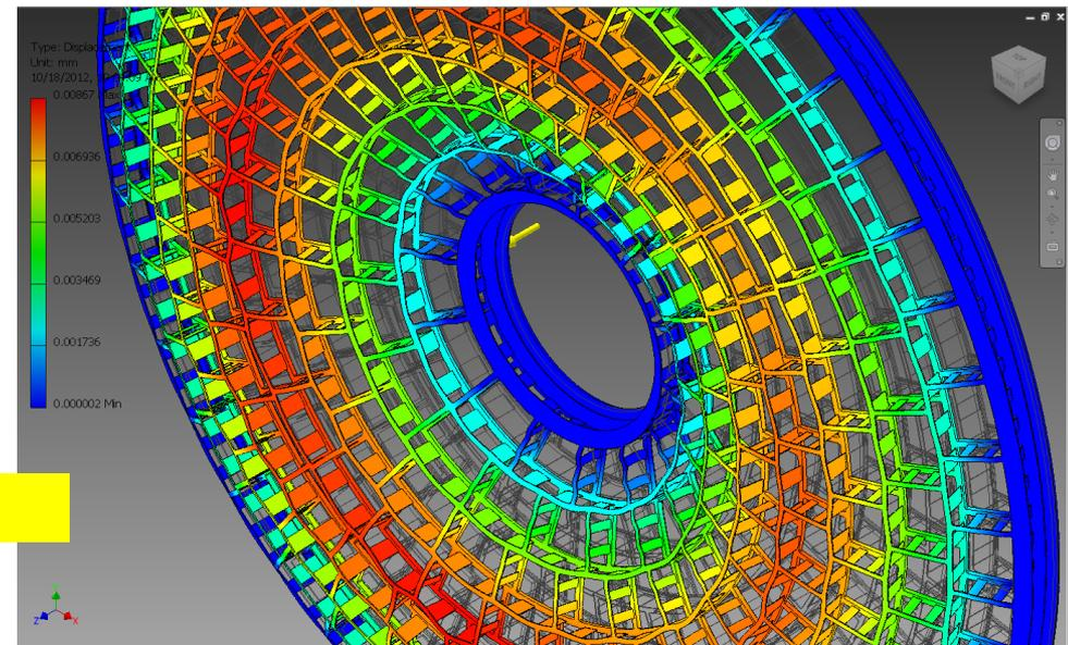
In the 4-row design, local distortions of 44 microns (0.002mm/100 N) can be seen in the back-disk.
