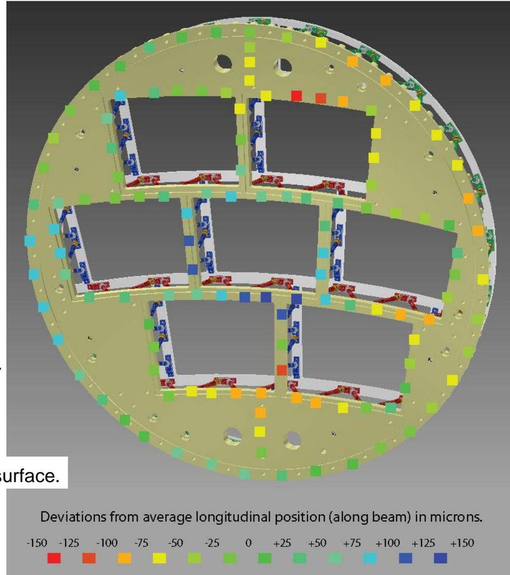
Deviations from average longitudinal position (along beam) in microns.
