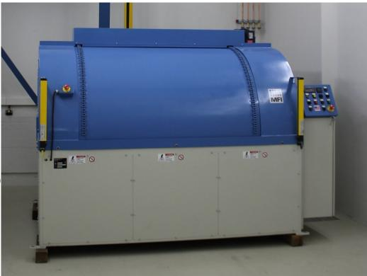
The machine is being commissioned based on the polishing recipes derived from best FNAL, JLAB, and previous DESY experience
