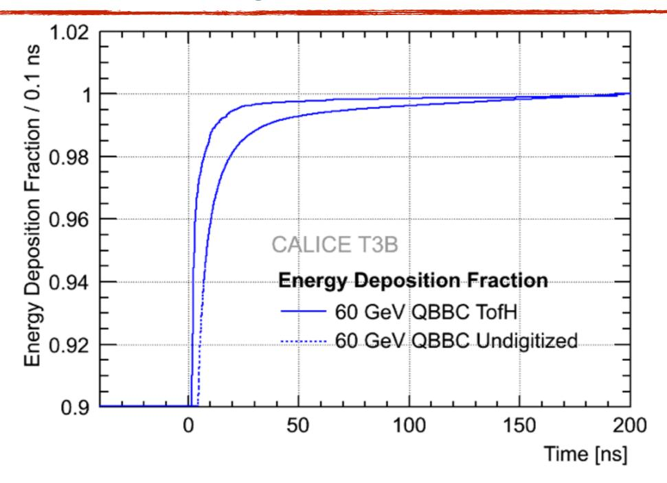
• Substantially faster integration with first hit only- but actually quite realistic in terms of a real detector (time stamp provided by start of signal in a cell, not by extension...)
