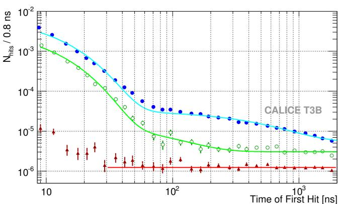
Fit with two-component exponential, to model the two different visually apparent time components:
