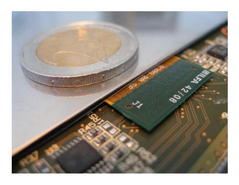
A flexlead disappears in an AHCAL steel cassette.
