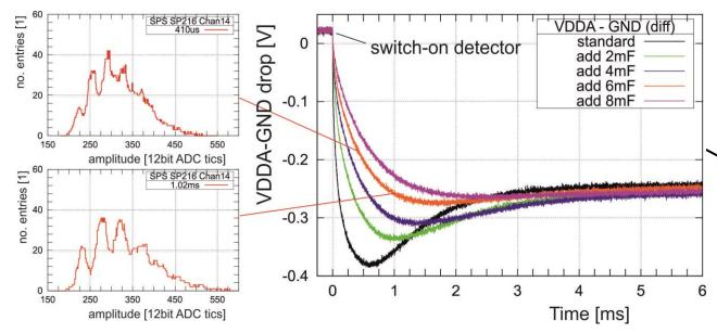
Switch-on time T\_on too small: Low gain and high noise!
