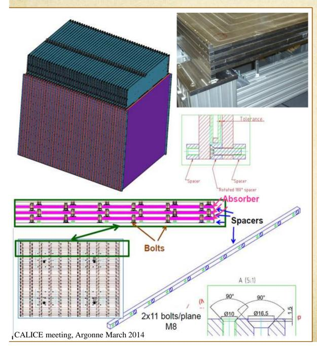
The 1m³ mechanical structure was made of 51 stainless steel plates assembled together using lateral spacers fixed to the absorbers through staggered bolts.
