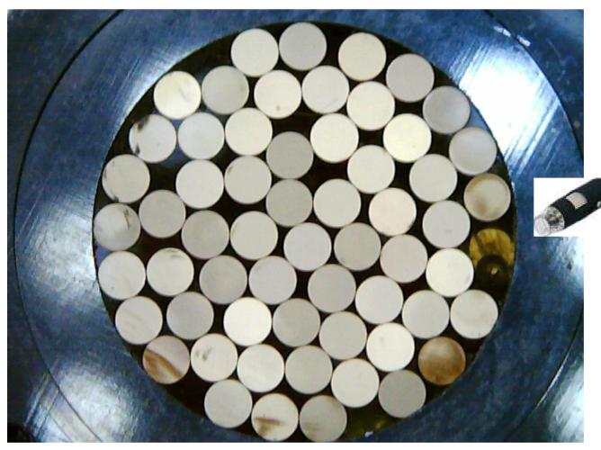
First picture of 60 of 1mm dia fibres illuminated by a daylight.
