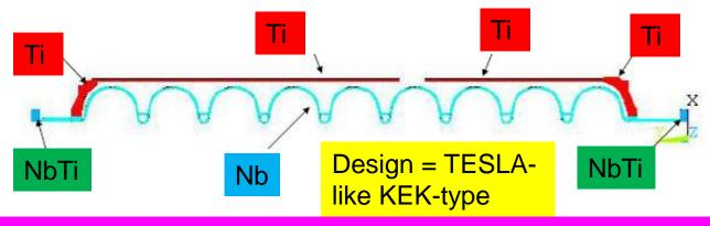
We must confirm the strength of liquid-He pressure-vessel by analysis with simulation and declare the welding details of Nb cavity and Ti jacket to the authority. In addition, we must perform series of pressure tests and report the results to the authority.
