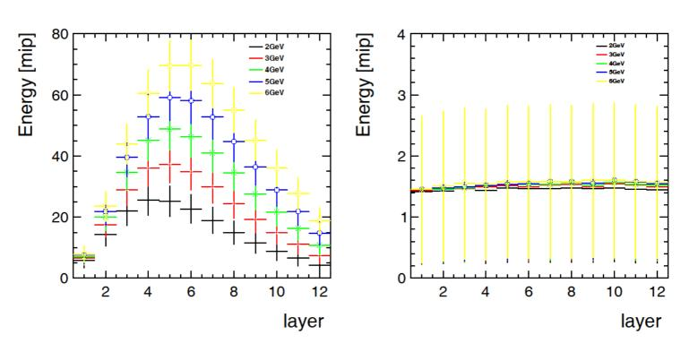
• Mean energy deposited per pad Electrons
