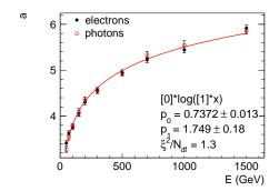
Dependence of the profile parameter a on the incident energy
