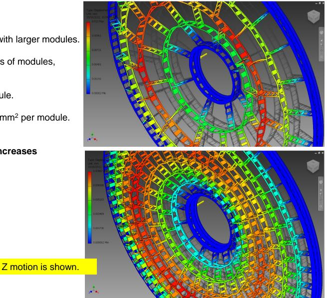
In the 4-row design, local distortions of 44 microns (0.002mm/100 N) can be seen in the back-disk.
