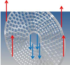
Endplate is supported at 4 points (*red arrows*) upper points are constraints, right fixed, left sliding lower points are forces
