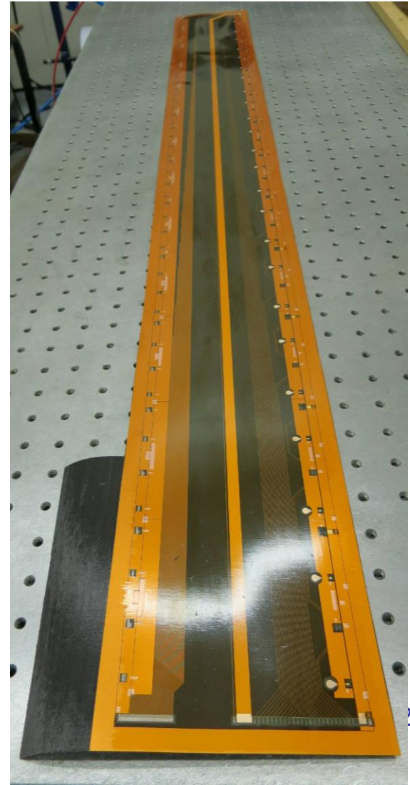
Cu/Kapton tape co-cured with K13C2U
