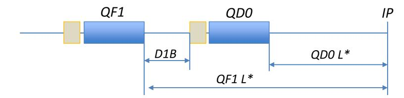
Bandwidths for optimized optics (not only strength of quad, but also quad location)
