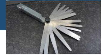
A fast quality control has been performed during the tests at ARKU using feeler gauges
