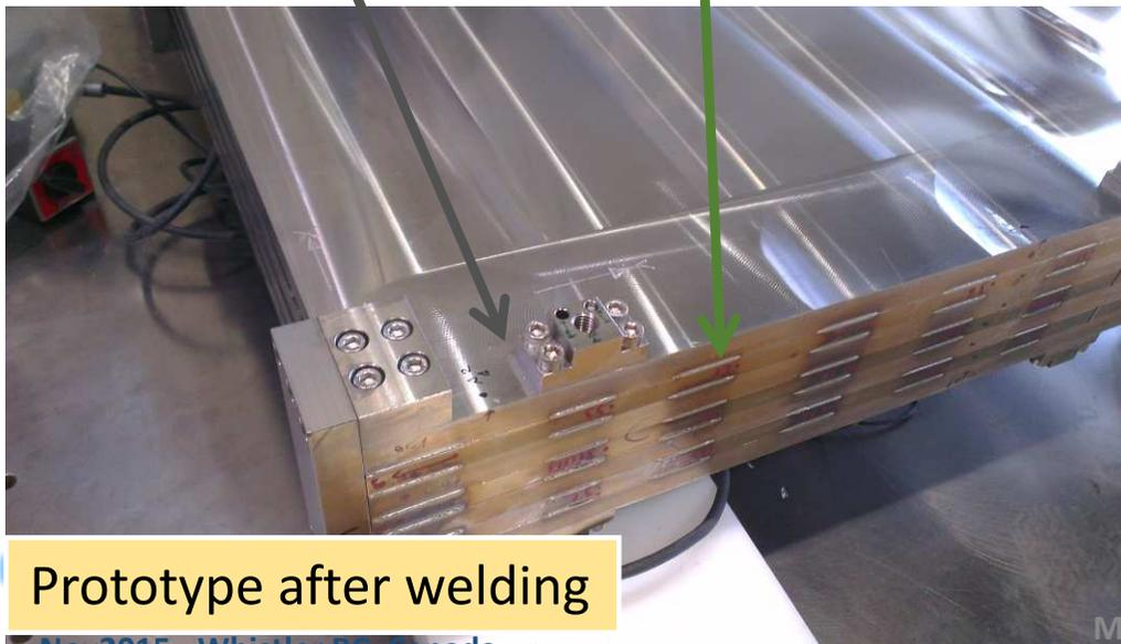
After comparing the measurements before and after welding deformations found (~1mm) bigger than expected in X-axis. O.K in Y-axis
