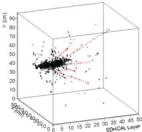
The tracks extracted from showers can be used for calibration, using them (requiring good tracks with good  $\chi^2$ ) to check the **efficiency** and **multiplicity** of the individual GRPCs
