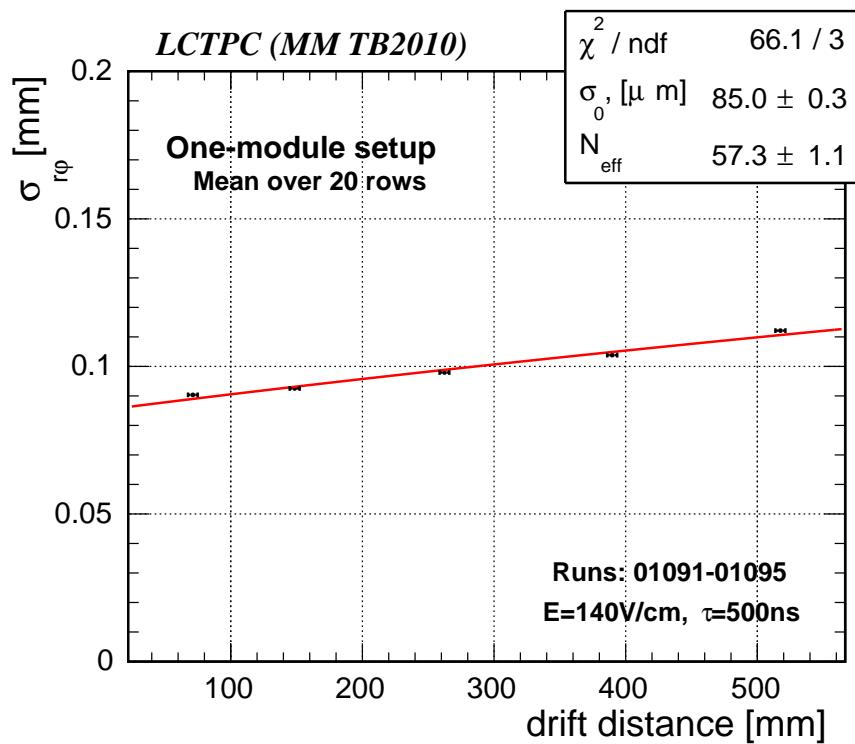
Reach about  $\sigma_{r\phi} = 110\mu\text{m}$  at large drift distance (very high  $N_{\text{eff}}$ )
