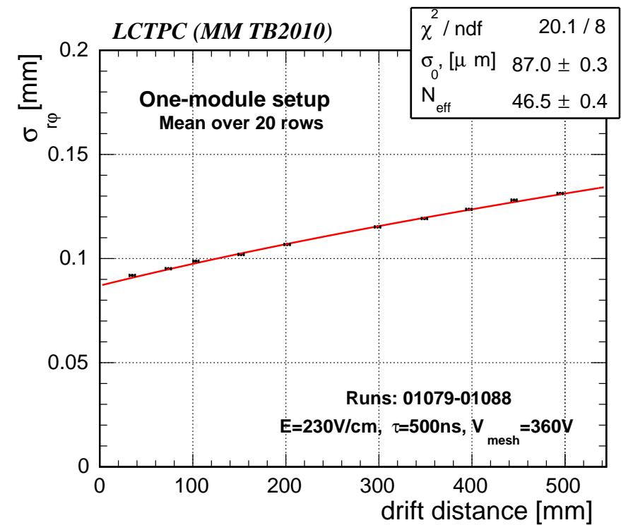
Lower gain degrades resolution at small drift distance (increase  $\sigma_0$  and  $N_{\text{eff}}$ )
