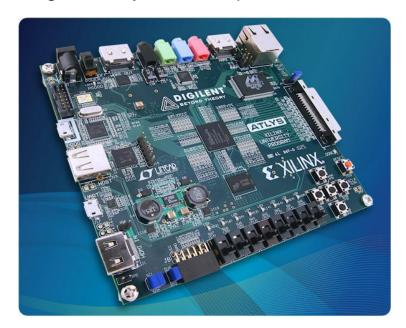
It can be communicated by Ethernet, USB, HDMI interfaces
