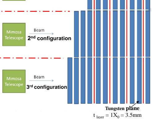
LumiCal sensor planes, 32 active channels/plane
