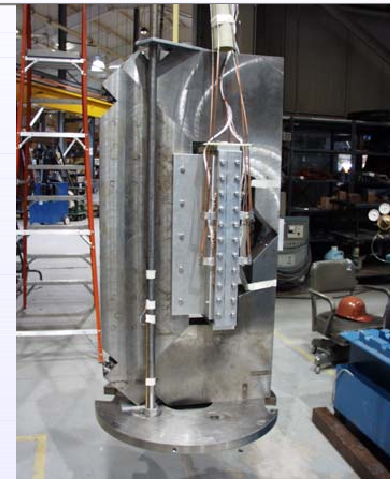
Cold iron magnetic mirror test with six coils
