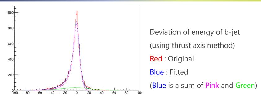
To estimate the b-jet energy resolution we use multiple Crystal Ball functions for fitting.
