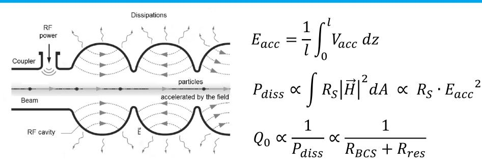
**D** Quality factor  $Q_0$  as figure of merit for the loss ( $\lambda_L = 47$ nm)
