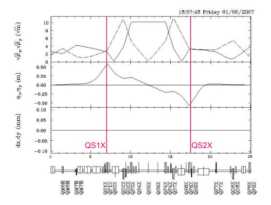
Candidate location of skew quads for vertical dispersion correction.
