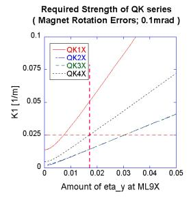
Amount of the correctable residual dispersion with IDX skew quads to QS1X and QS2X is 17mm.
