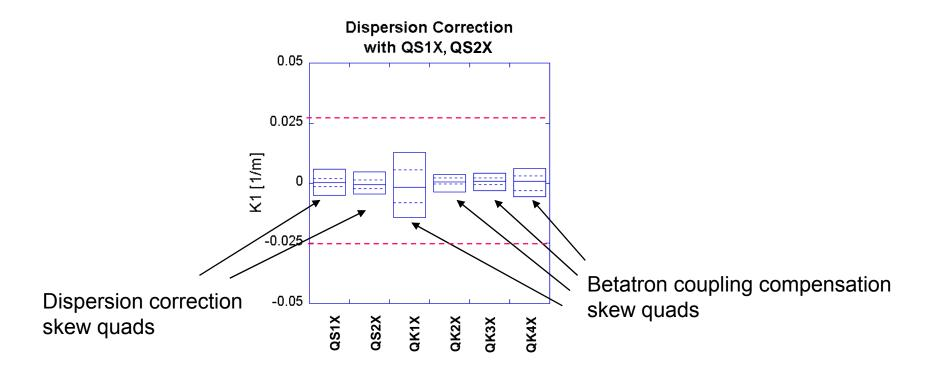
All of the skew strengths are within the strength of IDX skew quads.
