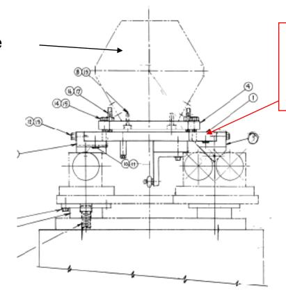
Put extra plates to lift up magnet as it does not fit between the shafts
