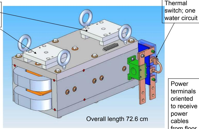
terminals oriented to receive power cables from floor
