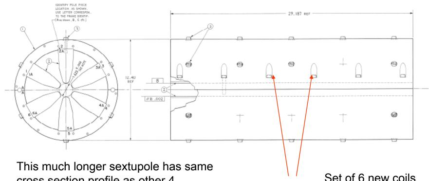
This much longer sextupole has same cross section profile as other 4 sextupoles, we will saw out a section of its core and mill the ends to make a 89.66 mm long core. The poletips will be machined back to 50mm diameter
