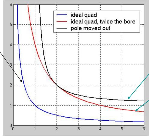
This section of the poletip is "missing" more material than it would if the pole had been machined back. This leads to higher 12-pole content in the shifted case.
