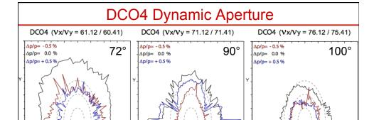
These dynamic aperture plots show the maximum initial amplitudes of stable trajectories. It is customary to overlay either the injected or equilibrium beam size on the plot. Significant margin is usually desirable in a design because machine errors (which cannot always be included) will degrade it.
