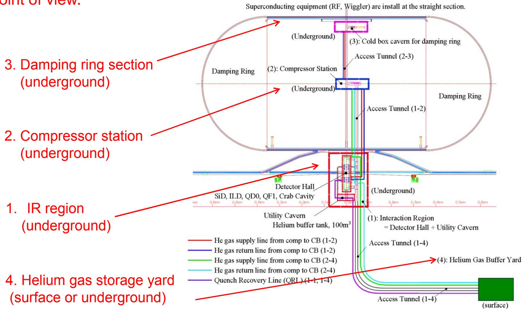
3. Damping ring section (underground)
