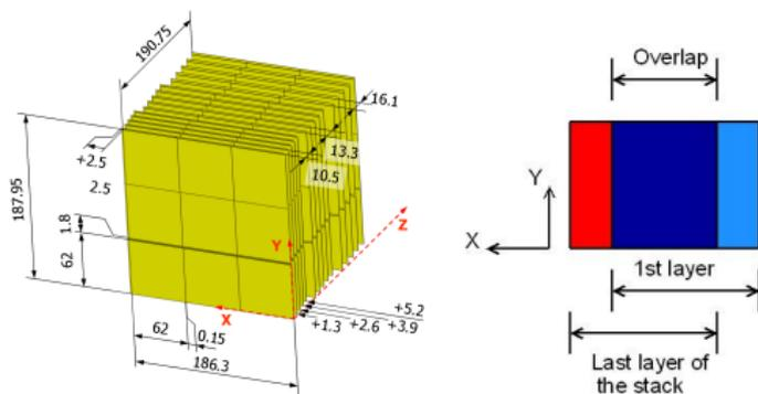
**Figure:** Picture of the ECAL layers' showing the staggering and drawing of the cut used
