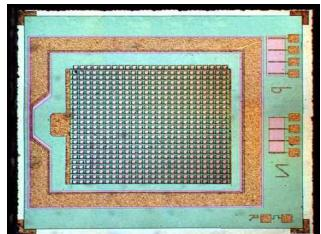
➍ 1156 pixels ( $30\times 30\text{ }\mu\text{m}^2$ ) per SiPM:
