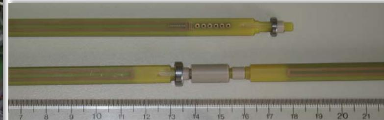
**“Single Stretched Wire”**: well known method: utilized for Gdl and magnetic axis measurements
