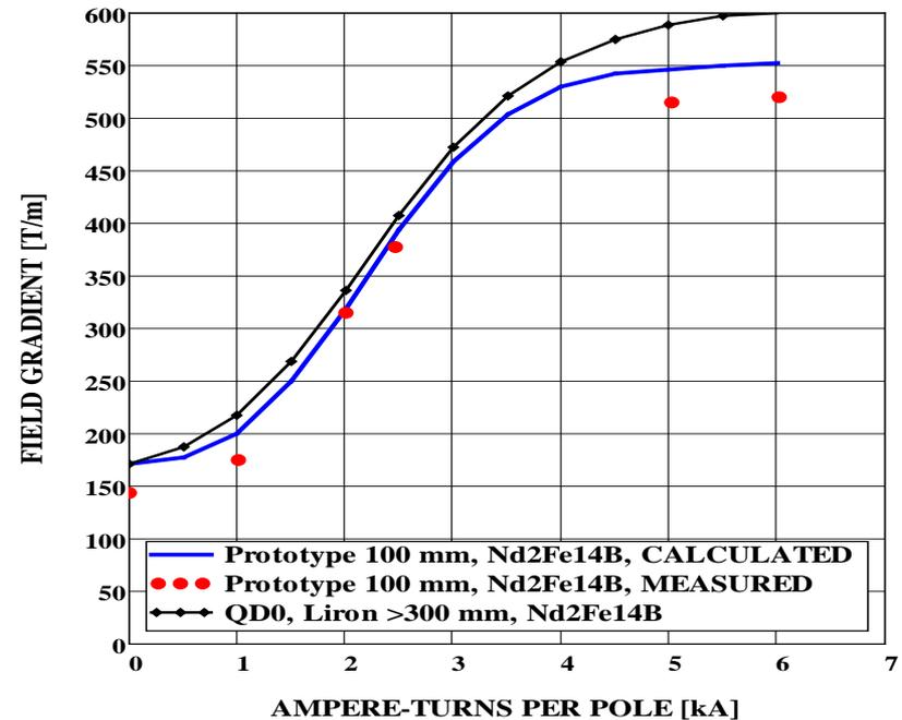
The measured Gradient in the configuration with  $\text{Sm}_2\text{Co}_{17}$  blocks (left) is in very good agreement with the FEA computation. This is not the case for the  $\text{Nd}_2\text{Fe}_{14}\text{B}$  blocks (right) where a difference of ~ 6% at maximum gradient is visible. This could have 2 possible explanation (the 1<sup>st</sup> was excluded by a further FEA cross-check):
