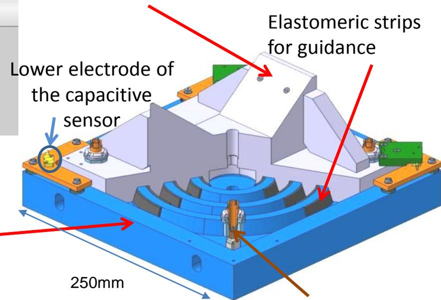
Additional passive stage directly under active system is also envisaged
