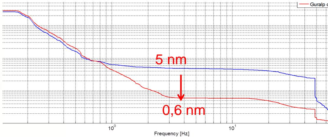
RMS ground at 4 Hz: 5 nm
