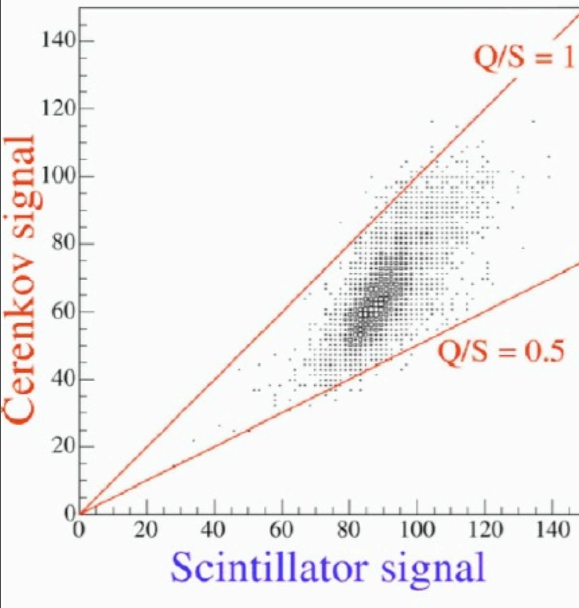
The DREAM “money plot”: the reconstructed energy given by the scintillator signal can be improved with the Cherenkov signal (e.m. component) since the slope of the distribution is  $\neq 1$
