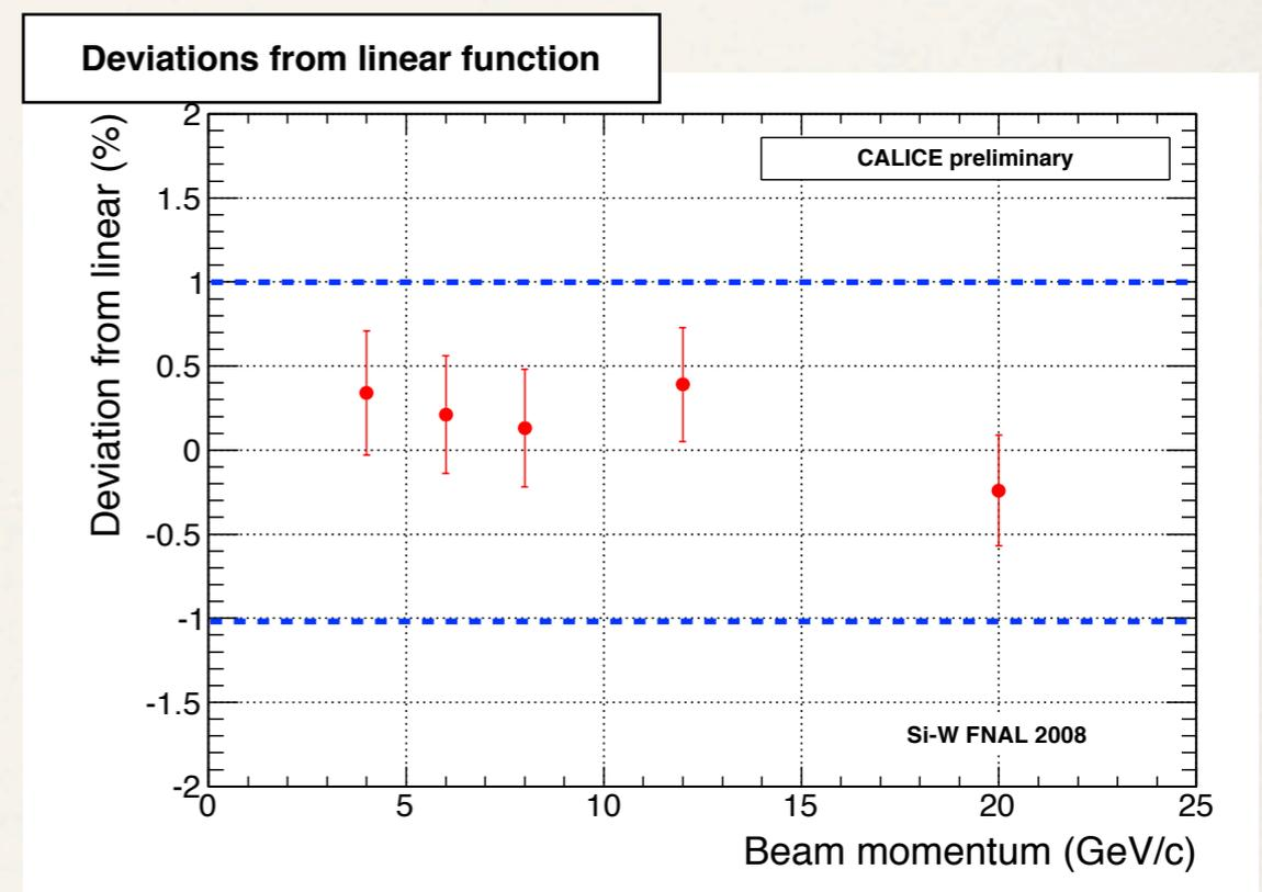
The deviations from linear function are less than 1 %
