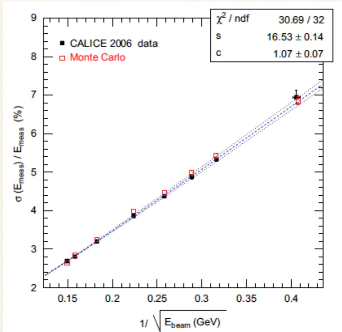
$$\frac{\sigma(E_{\text{meas}})}{E_{\text{meas}}} = \left( \frac{16.53 \pm 0.14(\text{stat}) \pm 0.4(\text{syst})}{\sqrt{E(\text{GeV})}} \oplus (1.07 \pm 0.07(\text{stat}) \pm 0.1(\text{syst})) \right) \%$$
