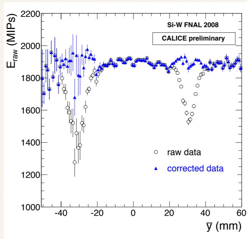
The energy loss in the inter wafer gaps can be corrected by applying  $1/f(\bar{x}, \bar{y})$  correction factor.
