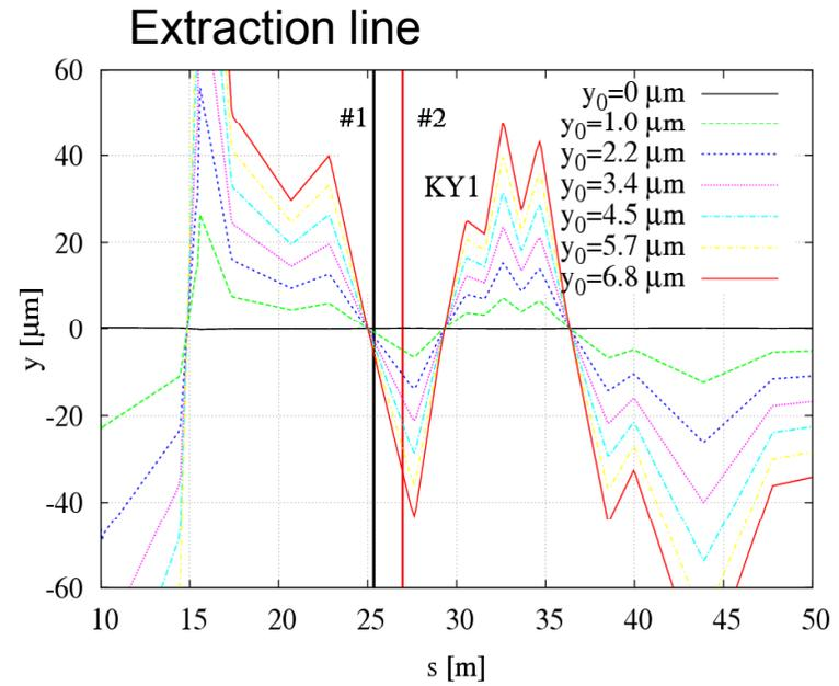
Example of a study of the effect of an initial vertical jitter in the range  $[0-7] \mu\text{m}$  and its transport to the IP
