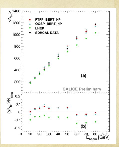
Although the digitizer is hadron-tuned one, for the tracks of the shower this should not be an issue. This was checked by putting d=0. The variation observed in the tracks number was found to be negligible. Thus, one can use the HT tracks to compare the hadronic shower models using variables
