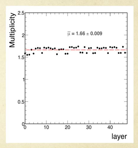
Muon efficiency and pad multiplicity in the simulation
