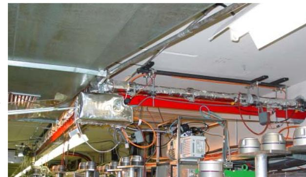
17m waveguide with 5 bends but low-loss (85% transmission) (Russian collaboration)
