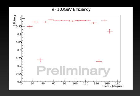
Electron Identification at higher energy slightly worse than tracking efficiency Transition region needs optimization
