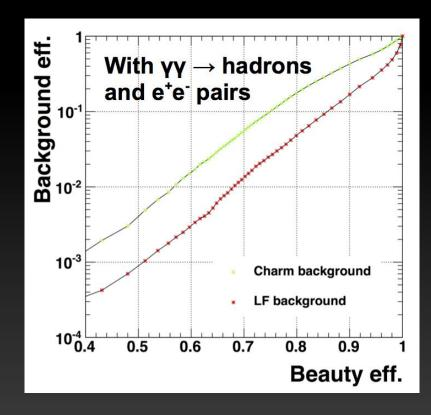
Using LCFIPlus, tuned for SiD detector Classifier trained on dijet events
