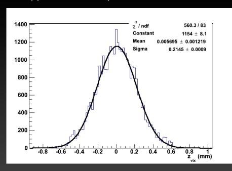
Fitted width: 214 µm
