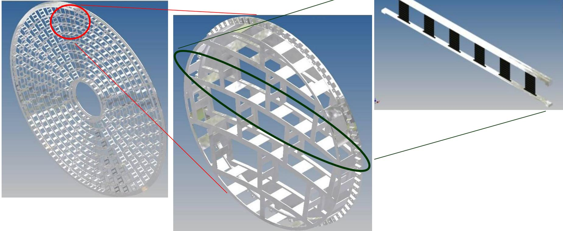
The ILD endplate design study involves endplates at 3 levels of scale.
