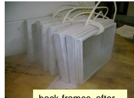
back-frames, after liquid N<sub>2</sub> immersion
