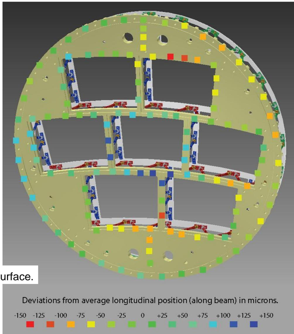
Deviations from average longitudinal position (along beam) in microns.
