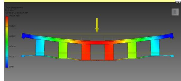
(Carbon fiber material is specified to have the same rigidity as the aluminum and is treated as aluminum in the FEA.)
