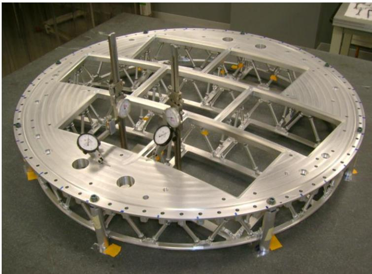
Note: in the original alignment, the inside surface is held on a flat surface, the outer disk was aligned to the specified height.
