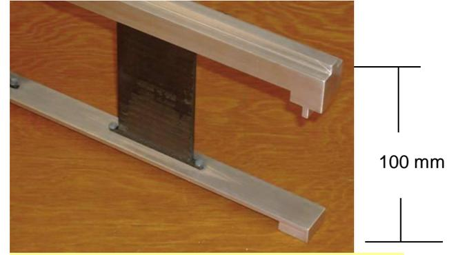
plate space-frame (carbon fiber)
